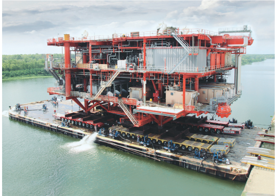
Transport of an offshore module weighing more than 1,000t using eight different Goldhofer self-propelled units.
